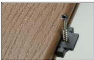
The Stowaway™ Hidden Fastener discreetly secures deck boards to joists with a single stainless steel, color-matched screw. The Stowaway screw comes preloaded, making the installation process faster, saving time and money. This system results in a beautiful, smooth and virtually fastener-free deck surface. Deck boards are automatically spaced at proper intervals, and the need for predrilling and countersinking are eliminated.
